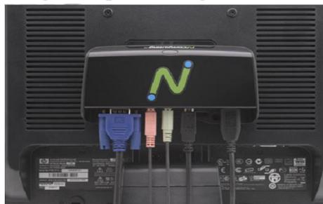
Gambar 5. Pemasangan NComputing di Belakang layar Monitor LCD
