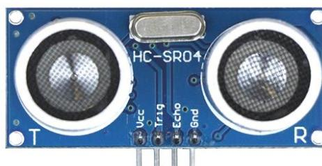
**Gambar 5.** Sensor sonar HC-SR04
