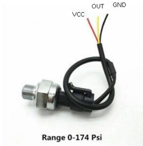
Gambar 10. Rangkaian Pressure Transmitter
