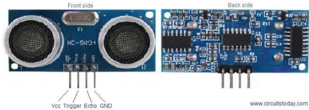
Gambar 2. Sensor Ultrasonik HC-SR04 (Sumber: https://www.circuitstoday.com/ultrasonic-range-finder-using-8051 )
